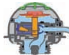
AutoMaXX with positive pressure – valve open
